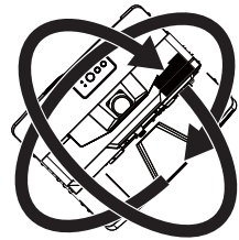
Tilt 360° (combination of horizontal and vertical)
